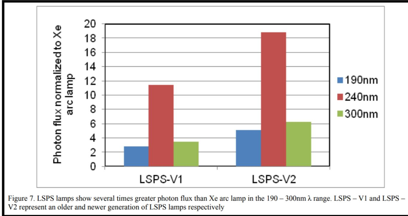
Figure 7. LSPS lamps show several times greater photon flux than Xe arc lamp in the 190 – 300nm  $\lambda$  range. LSPS – V1 and LSPS – V2 represent an older and newer generation of LSPS lamps respectively
