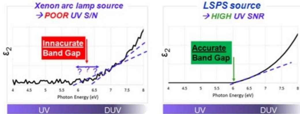
Figure 18. Bandgap of a material is estimated by the tangent to the  $\epsilon_2$  (obtained from dispersion) vs photon energy curve at the inflection point. The noisier the data, the more tangent solutions would be possible, thereby increasing inaccuracy
