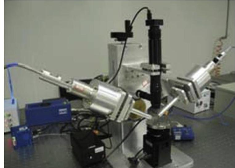
**Fig. 1.** Principle and prototype of the dual rotating-compensator Mueller matrix ellipsometer.
